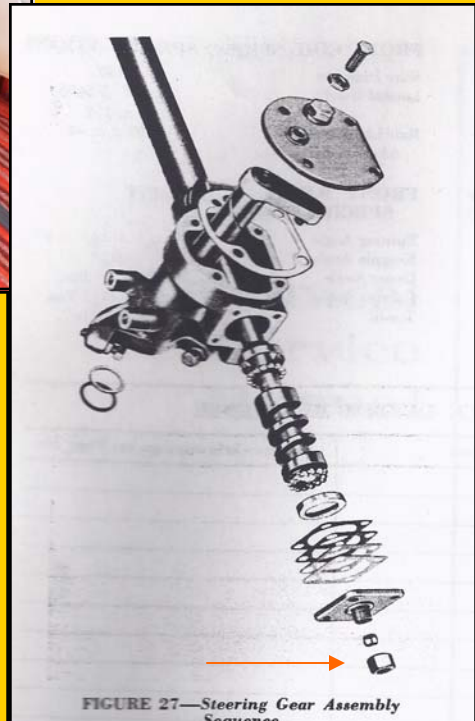
FIGURE 27—Steering Gear Assembly Sequence
